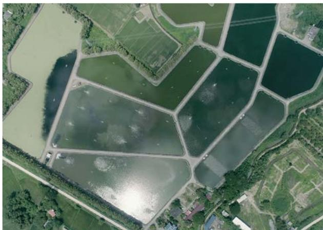
Aerated lagoons (AL) in Chiang Mai. This treatment method is typical for this region. ALs are easy and inexpensive to construct and operate. With this method, waste is degraded by various microbiological populations and pathogens can be effectively removed by aeration or exposure to sunlight. ©GIZ
